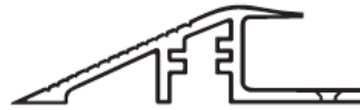
Aluminium ramping (for 14mm height grid only, with screws & rawl plugs supplied)
